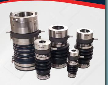
The Packless Sealing System (PSS) Shaft Seal is a mechanical face seal that is created between a rotating stainless steel rotor and a stationary carbon stator. The carbon stator is attached to a convoluted rubber bellow and the back of the bellow is attached to the shaft log (stern-tube) of the boat with hose clamps.
